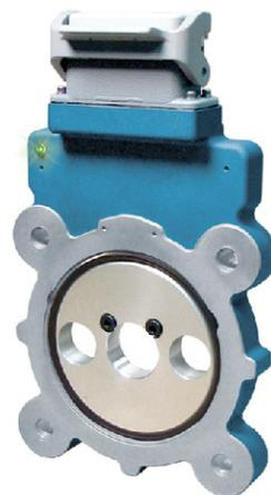
**A2:** Use fully potted encoder models with superior seals. If the electronics are fully potted into a brick of plastic, even if contamination enters the encoder, it can't harm the electronics. By using a superior seal, abrasive particles can be kept out that could otherwise harm encoder bearings. Again, no-bearing models are even better, because they don't have bearings to protect.
