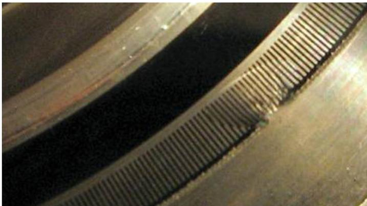
**1. Rough handling or installation.** The glass disks and precision optics used in optical encoders were designed for precise machine tools, not banging up 80m towers on a tool belt while climbing a ladder or
