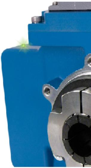
**A3:** Add predictive encoder diagnostics. Predictive diagnostics can be added to the encoder to indicate when the signal is less-than-ideal. Both local indication for the service technician (LED), and remote indication for the site manager should be provided. If an encoder reaches its signal limits, it issues a warning before it causes a shutdown of the turbine. The encoder can be accessed and serviced during scheduled downtime.
