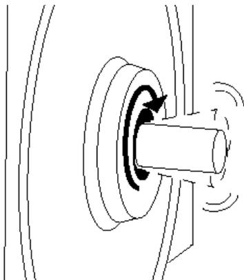
2. Rough installation. If a hollow shaft encoder is pounded on the shaft even by hand, this damages the encoder bearings. Failure is not immediate, but the encoder is doomed.
