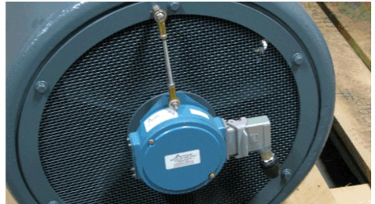
4. Undersize encoder bearings. Many encoders use tiny bearings (<100lb rating), and this makes them extremely vulnerable to items (1-3).
