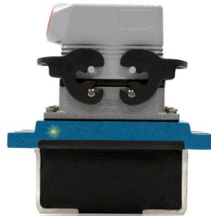
**A1:** Use a heavier duty magnetic encoder. Magnetic encoders don't have the precision optics that are vulnerable to rough handling. Heavy duty models pot the electronics into a solid block of plastic, and protect them with a cast aluminum housing. With Wide-Gap technology, the sensor can be very far from the spinning rotor so even continuous vibration and heavy shocks can't cause the magnetic sensor to strike the rotor.
